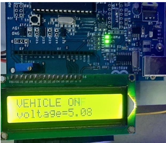
FIGURE 12: EV ON AND CHARGING AT 5V
