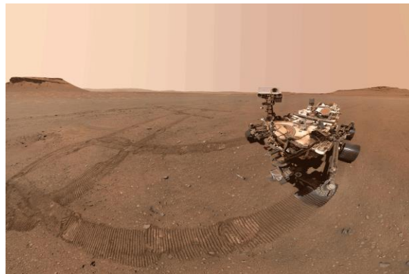
Figure 1: The Perseverance Rover used an intelligent targeting software, Autonomous Exploration for Gathering Increased Science system (AEGIS), which selects and targets rocks using the remotely controlled SuperCa
