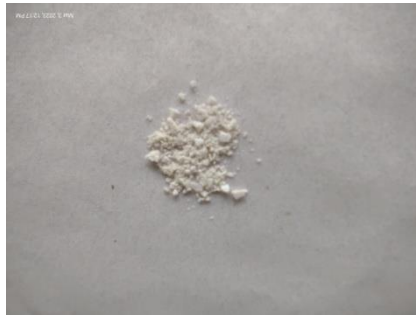
Fig. 11. Powdered amorphous silica, the root cause of white layer deposition on basaltic rock surface, being the dead debris/dead remains of diatoms.
