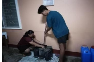
Figure 2.3.3 Applying 25 blows in every layer
