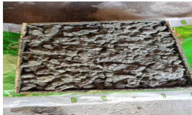
Figure 2.3.4 A 12"x12"x4" block, used for testing the infiltration
