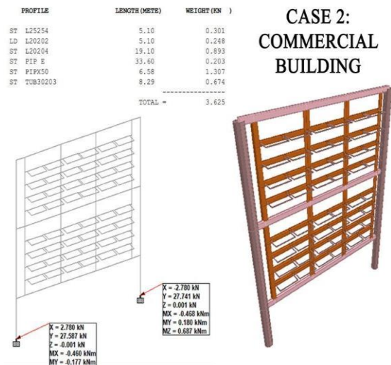
Figure-18: Design and Load Calculation from STAAD for Case 2
