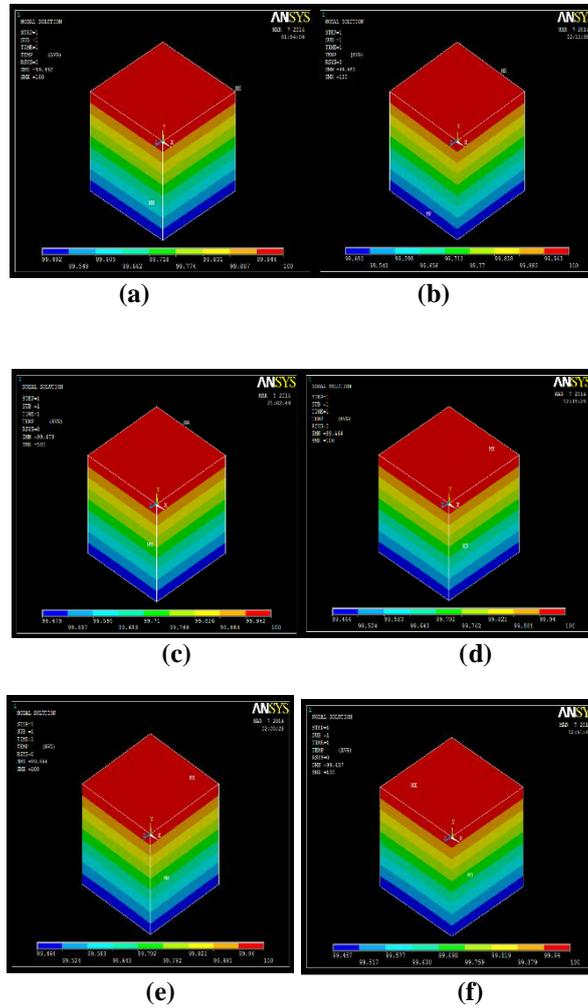
Figure 9: Temperature distribution of composites with glass fiber loading (a) 2.83 percent by volume (b) 5.65 percent by volume (c) 7.54 volume percent (d) 10.05 volume percent (e) 12.56 volume percent (f) 15.7 volume percent
