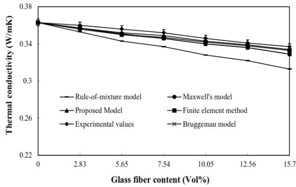
Figure 11: Thermal conductivity of short glass fiber/epoxy composites: Maxwell's model, Bruggeman model, proposed model, FEM, and experimental values
