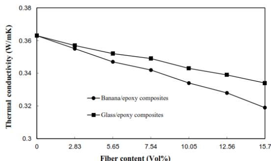
Figure 13: Correlation of the  $K_{eff}$  measurements for both the reinforcements (Proposed model)
