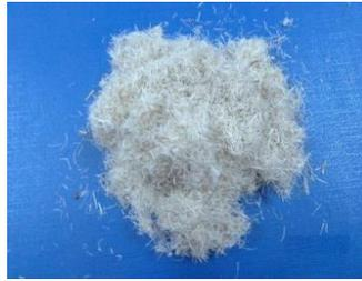
**Figure 5: Short banana fiber used as filler in the present work**
