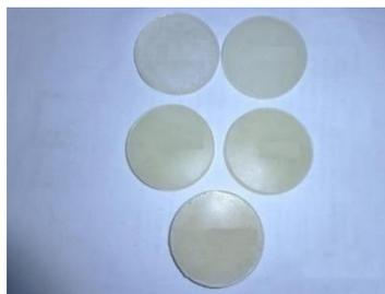
**Figure 6: Short glass fiber reinforced epoxy composites**
