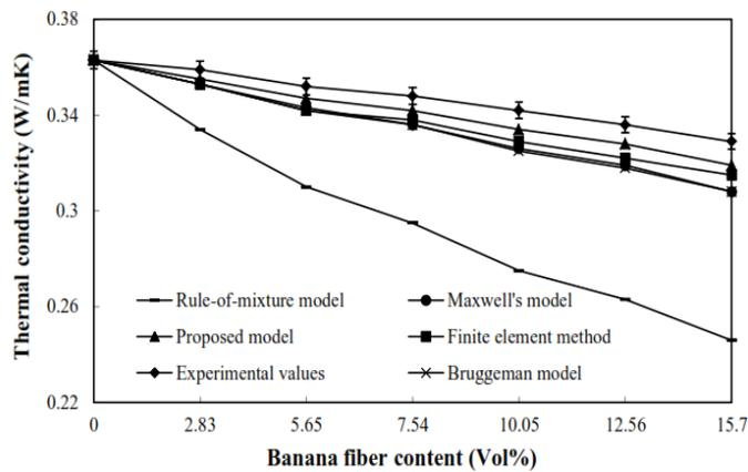
Figure 12: Thermal conductivity of short banana fiber/epoxy composites: Maxwell's model, Bruggeman model, proposed model, FEM, and experimental values
