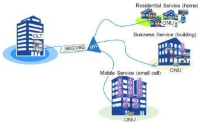
Fig. 1. Future high-capacity and low latency PON accommodating mobile, business, residential services in a single ODN
