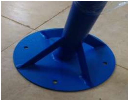
Fabrication of stiffener on stand
