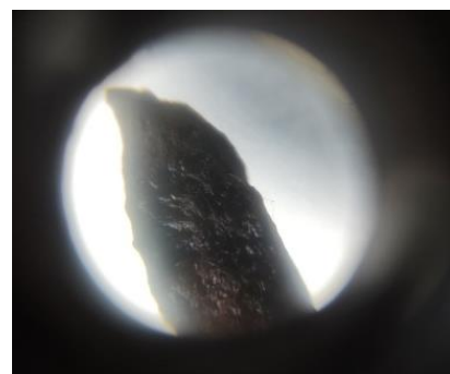
Fig. 8 Nantan stony iron meteorite observed through student microscope of 20x. The burnt and the rusting part is clearly seen
