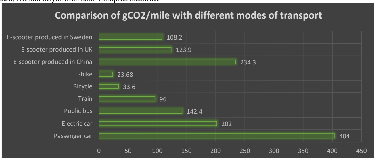
Figure 9 comparing the per mile emissions of the e-scooters from different production locations with other modes of transport – refer to sources [37] for figures on e-bikes and bicycles, [38] for figures on public buses and trains in the UK and [31],[30] for figures on electric and passenger cars.
