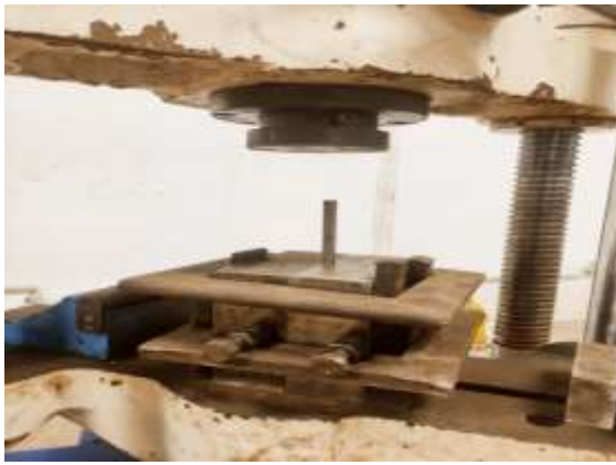
Fig 2.2.2 Die Set Up On Utm
