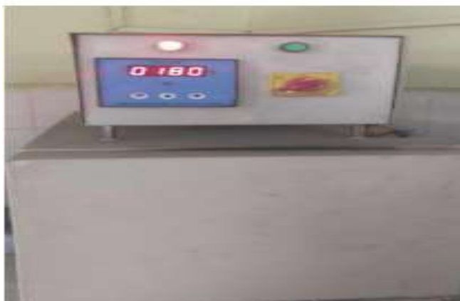
Fig 2.3.1Furnance used for aging and quenched in water
