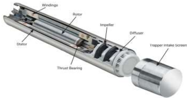
Figure 3: 3D render of STP Motor Assembly
