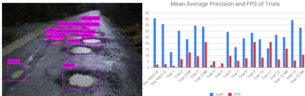
Figure 7: Potholes detected by yolo algorithm
