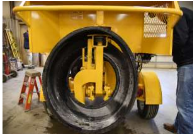
Figure 1: Tire Side Wall Cutter Machine
