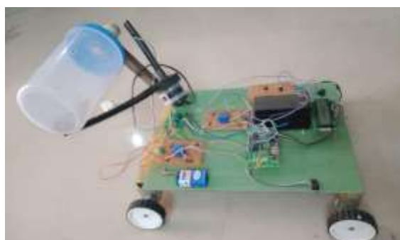
Fig-1 Working Prototype of automatic seeding and pour water robot for Agriculture
