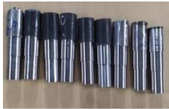
Image 8: Work specimens after turning
