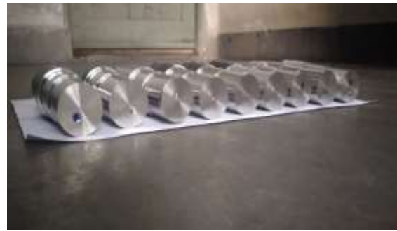
Image 9: Work specimens after surface hardness testing
