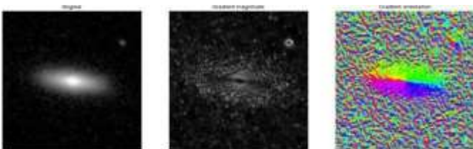
Fig 4(a): Original Image. (b): Gradient Magnitude of the Image. (c): Gradient Orientation in HSV colormap.
