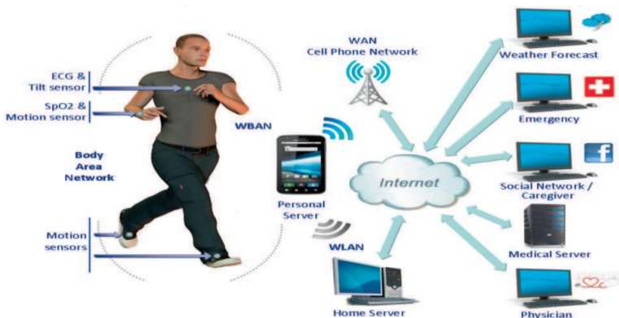
Figure 2.1 System Architecture of The Ubiquitous Health Monitoring System
