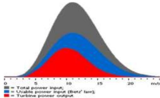
Fig.3: Power Density Curve
