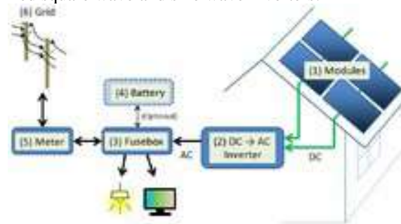
Figure 5 : working layout of solar inverter
