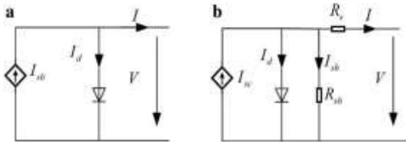
Fig.1a and Fig. 1b are ideal and practical circuits respectively
