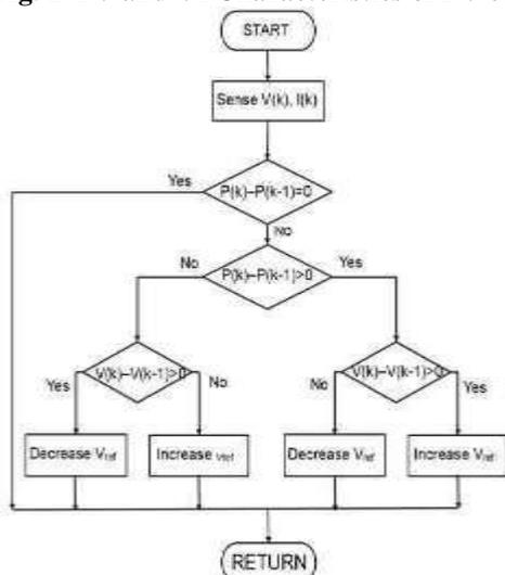
Fig. 3 flow chart of P&O algorithm
