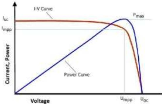
Fig. 2 PV and VI Characteristics of PV cell
