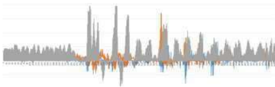
Fig 6.2 – High Frequency oscillations For Pothole
