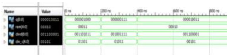
Fig. 3 Simulation result for division of 8-bit binary numbers using Vedic mathematics sutras
