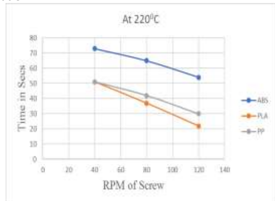
Graph 4.6 indicates the time verses various speed of screw at same 220 0 C temperature of ABS PLA and PPmaterials.
