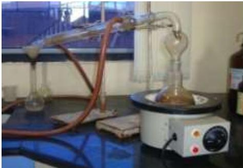
Figure 5: Distillation and recovery of alcohol (Figure from Author)
