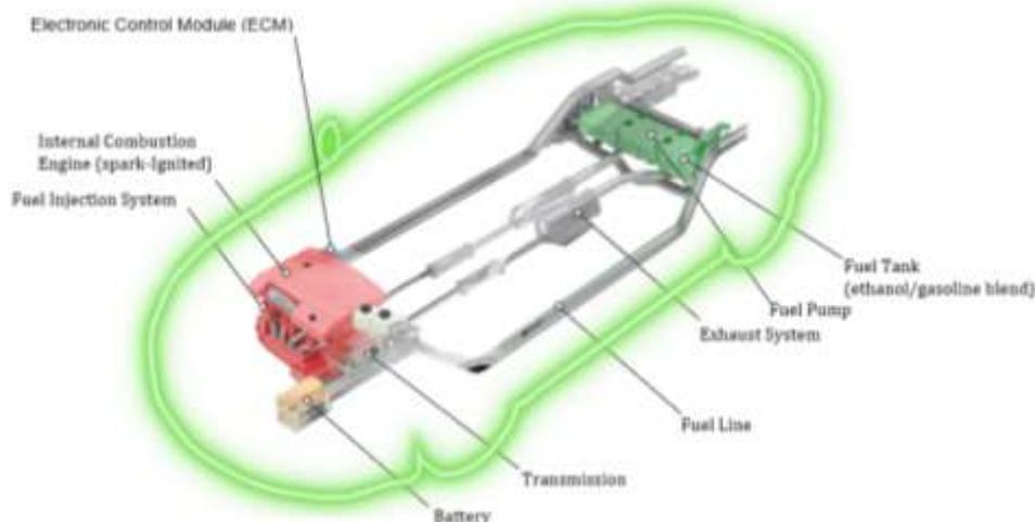
Figure 7: Flexible Fuel Vehicle
