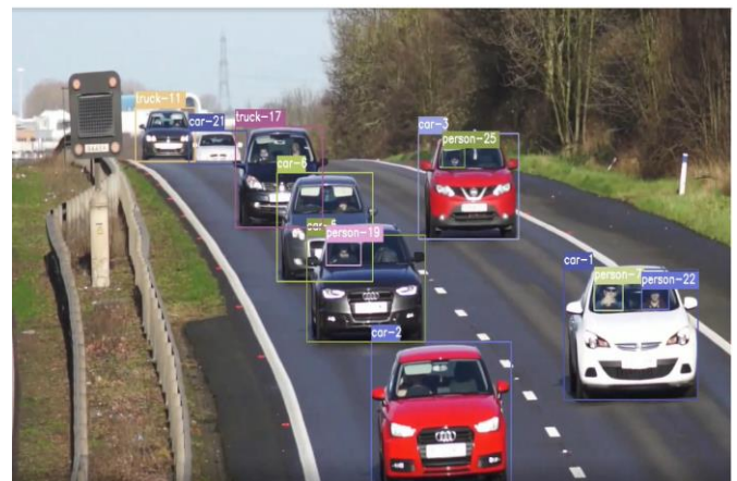
Figure 6 – Object detection and Tracking using YOLOv4 and Deepsort on Cars Dataset
