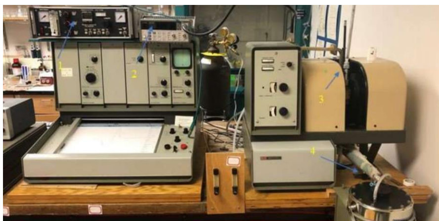
Figure 4: Setup of the Varian E-3 X-band spectrometer used for the experiment.
