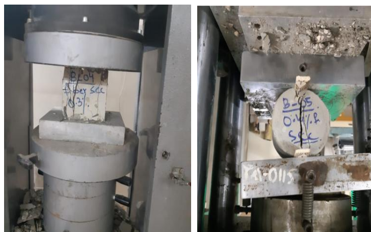
Figure 12. Pictorial view of cube and cylinder specimen at ultimate failure
