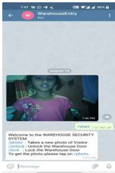
Figure : Initialize of Warehouse Door Monitoring
