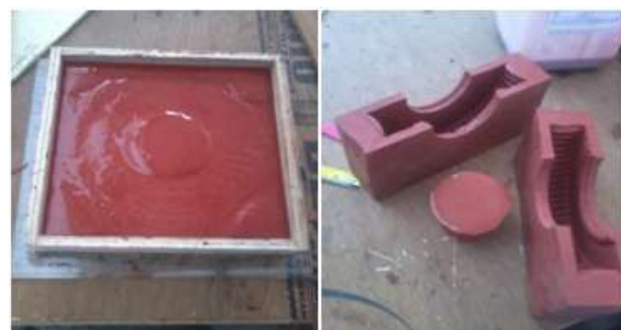
Figure 4.1 (b): - Curing of Rubber Mold And Split Mold
