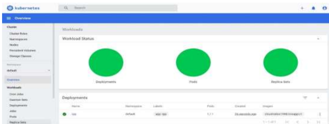
Figure - 11: Kubernetes UI Dashboard page (consisting of all the required details concerning deployment, pods)
