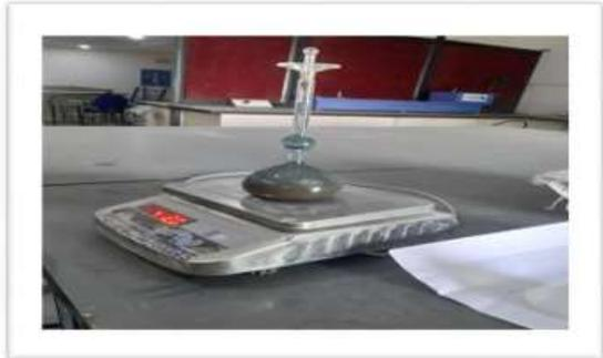
Figure.5 Specific gravity of cement
