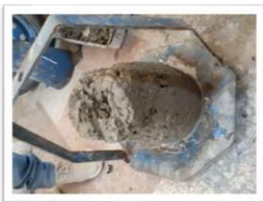
**Figure.10 Slump flow test**
