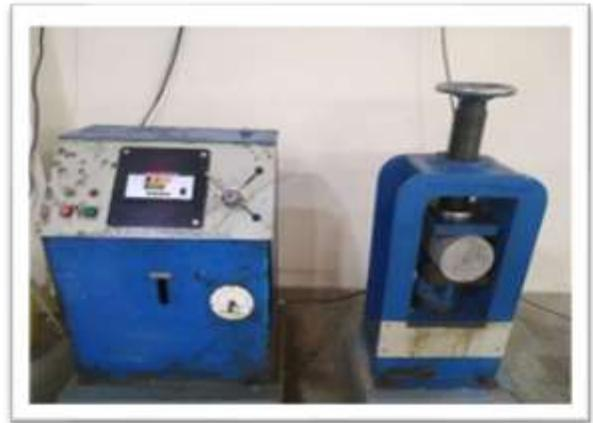
Figure 15 Split tensile strength using UTM
