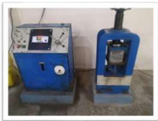
Figure 14 Compressive test using UTM
