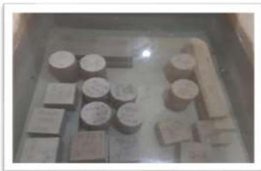
Figure.13 Specimen in curing tank
