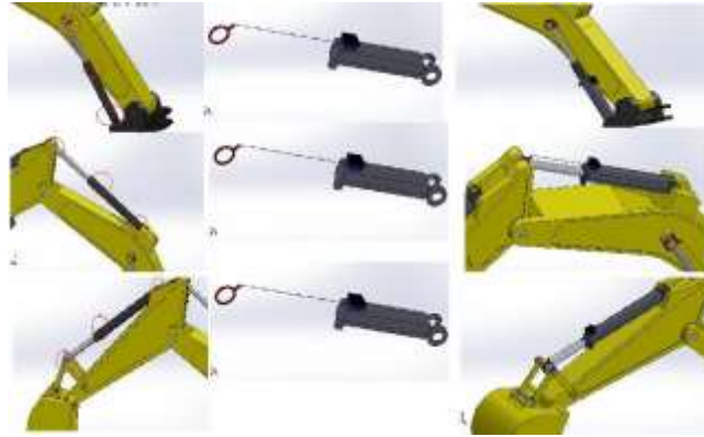
Fig6. column 1(from left) (from top wire sensor install location for boom,arm and bucket respectively) Column 2(from left)(Wire Sensor Design for boom,arm and bucket from top respectively) Column 3(from left)(Installed wire sensor for boom,arm and bucket from top respectively)
