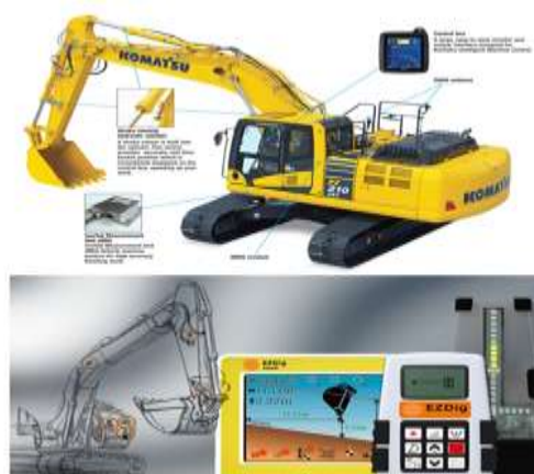
Fig1. (top) Machine guidance using measured cylinder length, which is developed by KOMATSU; (bottom) Machine guidance using measured links motion, which is developed by EZDig.
