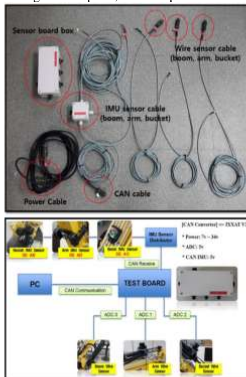
FIG8. Circuit connection Diagram
