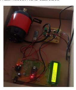
As described in the above chapters, the motor can be controlled using the mobile phone using the S2 Application. Five speeds are configured and each speed can administered by sending the respective character from 1 to 5 via the application. We can also monitor the temperature by sending the asterisk \* character
