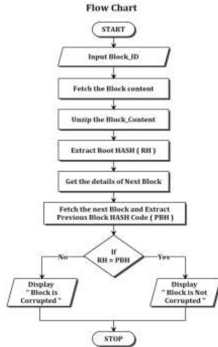
**Figure1 – Block validation flow**
