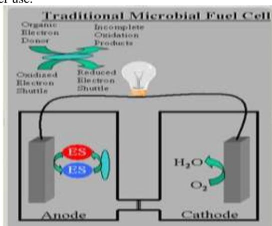
Fig. (1) Traditional Microbial Fuel Cells
