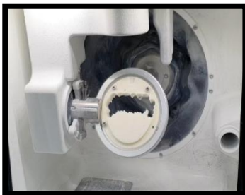
Cad milling machine for wax designs and final prosthesis ceramic designs.
