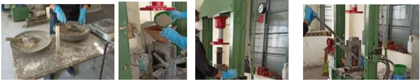
(a) Mixing of material (b) Placing in mould (c) Operating Hydraulic Press (d) Ejecting from the mould
