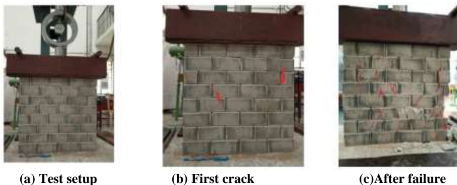
Fig. 8: Test on IB wall panel
