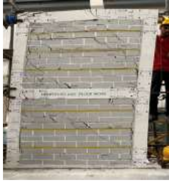
Figure-5: Deformed Reinforced Aerocon Block RC Frame
