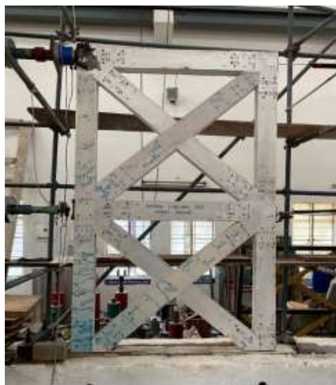
Figure-13: Deformed Double Diagonal RC Strut Frame
