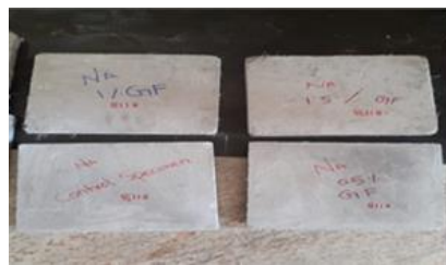
Fig. 3: Thermal conductivity plate specimen
