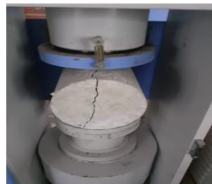
Fig. 2: Split tensile strength test
