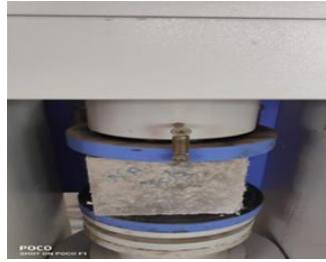
Fig. 1: Compressive strength test
