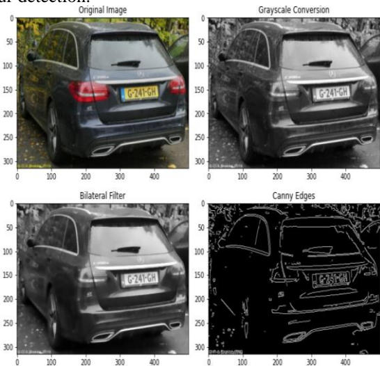
Fig 3. (a) original image (b) grayscale conversion (c) Bilateral Filter (d) Canny Edges
