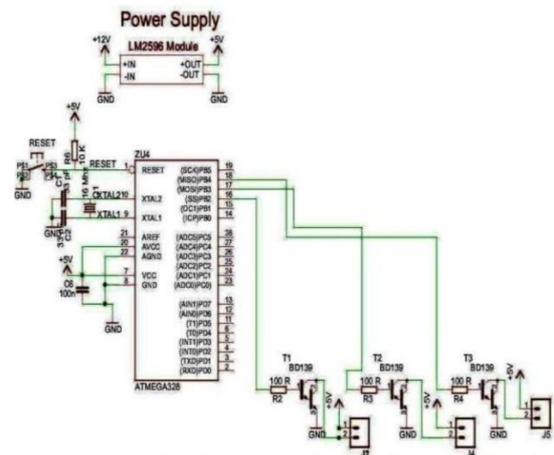
Fig. 3: Receiver Section
