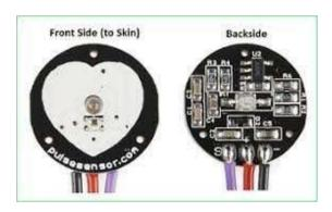
The Pulse Sensor is well-designed low-power plug- and play heart-rate sensor for the Arduino. This sensor plugs right into Arduino and simply clips onto a fingertip or earlobe.
