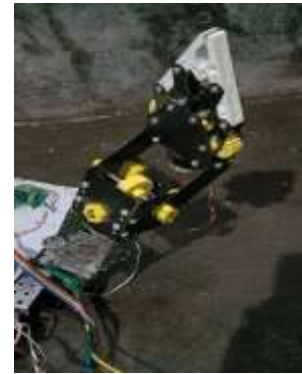
Fig-3: Rotatable Mechanical Gripper
