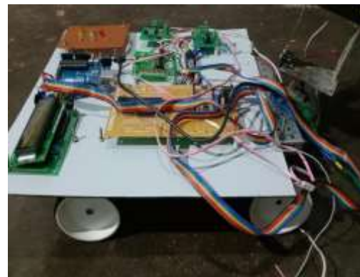
Fig-4: Hardware Connections on Wheeled Platform
