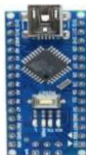
The Arduino Nano is a small, complete, and breadboard-friendly board based on the ATmega328 (Arduino Nano 3.x). It has more or less the same functionality of the Arduino Duemilanove, but in a different package. It lacks only a DC power jack, and works with a Mini-B USB cable instead of a standard one.
