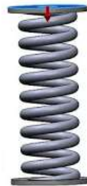
Fig-3.11 Helical Compression Spring
