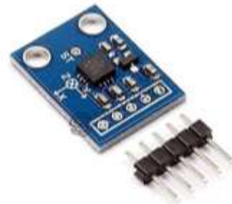
Fig-3.5: Accelerometer Sensor
