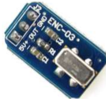
Fig-3,6: gyroscope Sensor
