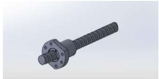
Fig-3.10: Re-Circulating Ball Screw Mechanism
