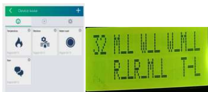
Fig.4: Normal condition of active sensors shown in mobile app and LCD display
