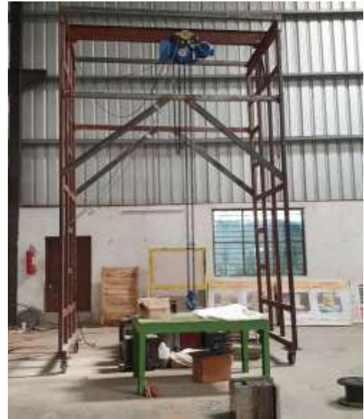
Mould lifting crane has been given no proper space
