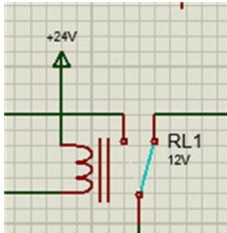
Fig 7(a): Relay deactivated when V < 12
