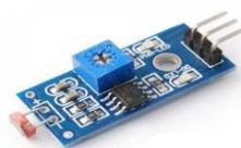
Fig-5: LDR Sensor
